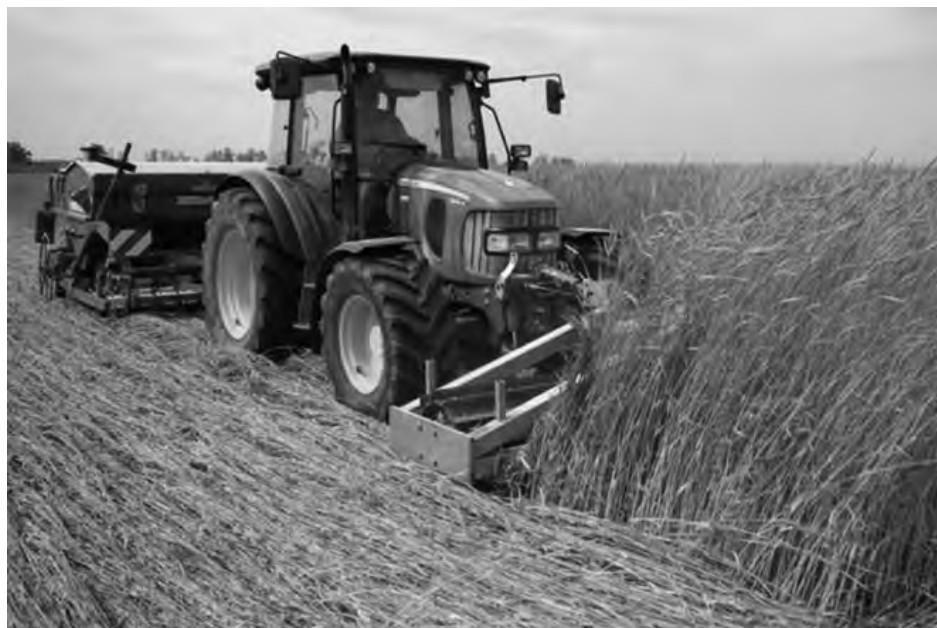
Figure 1: Rolling, crimping and seeding at once
